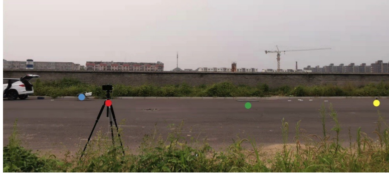
Figure 28: Experiment set up. The camera shooting videos from the side is marked with red dot. The camera shooting videos in front of the launcher is marked with yellow dot. The launcher is marked with blue dot, and the rubber plastic pad is marked with green dot.
