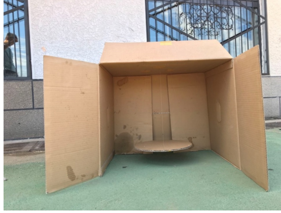
Figure 21: Measuring the period of oscillation of the lower board. The lower board is twisted with a small angle, and set free to oscillate.
