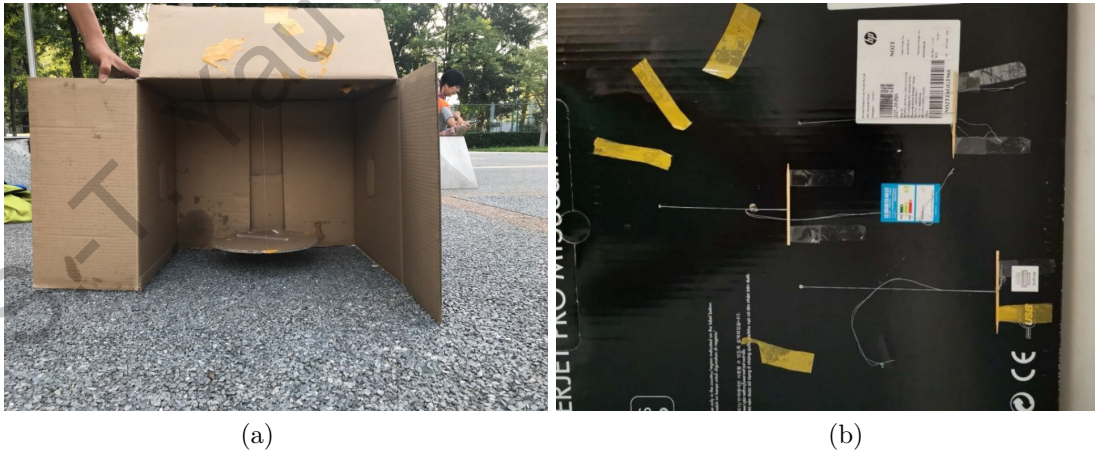
Figure 19: (a): Experiment setup for measuring moment of inertia. (b) Configuration of toothpicks and adhesive tapes. The tooth picks are fixed on the board, and the threads are tied on the tooth picks.
