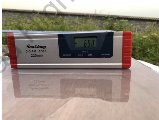
Figure 29: Electronic level used to measure the pitch angle established by the launcher
