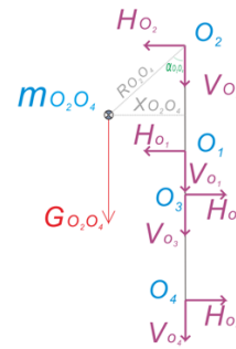
Figure 5. FBD of linkage O_2O_4 .
