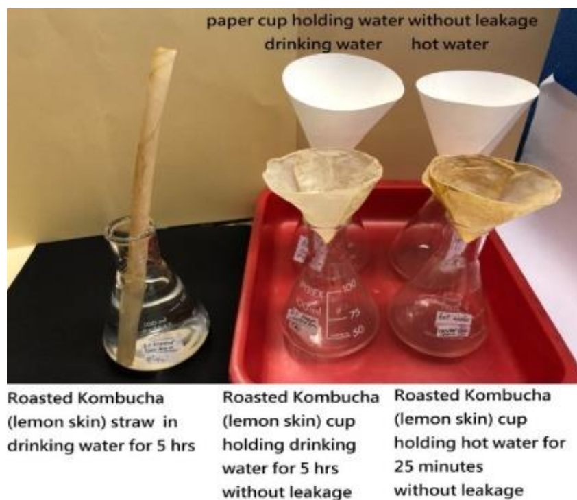
Fig.3.6.2.1 Performance of roasted kombucha cups and paper cups holding drinking water and hot water without leakage
