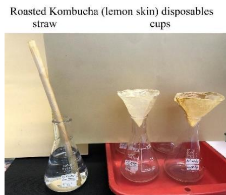
Fig.3.6.1 straw(left) & cups(right) made of roasted kombuchas of lemon skins
