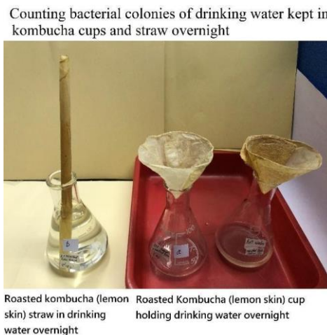
Figure 2.5.2 experiment set up about studying the growth of oral bacteria in drinking water
