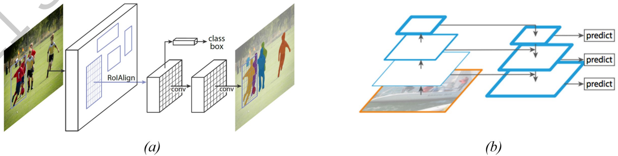
Figure 9: Mask R-CNN framework [22] (a) and FPN architecture [31] (b).
