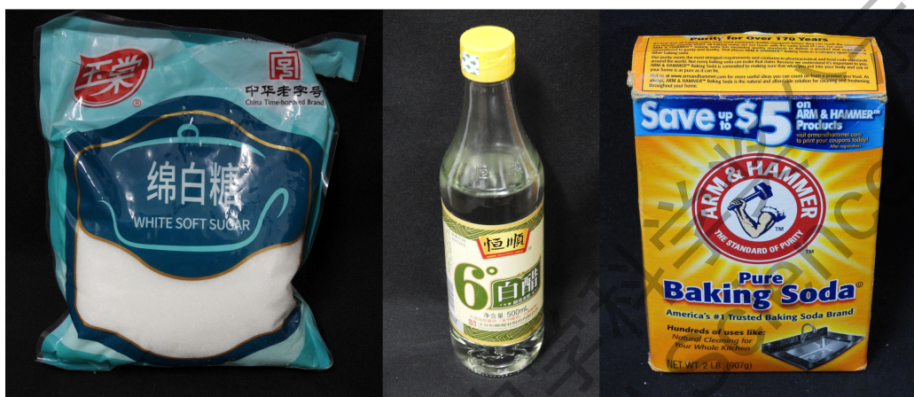
Fig 1 , The Materials used for CQD synthesis: Table Sugar/sucrose (Left); White vinegar (Middle); Baking soda/sodium bicarbonate (Right).
