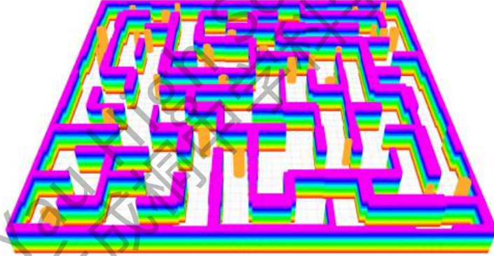
Figure 10: An example of a procedurally generated maze. The colored wall point clouds represent the maze geometry, while the orange cylinders denote dynamic obstacles placed in the free corridors
