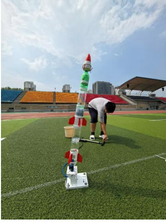
Figure 3-1. Water rocket experimental platform and sensor payload
