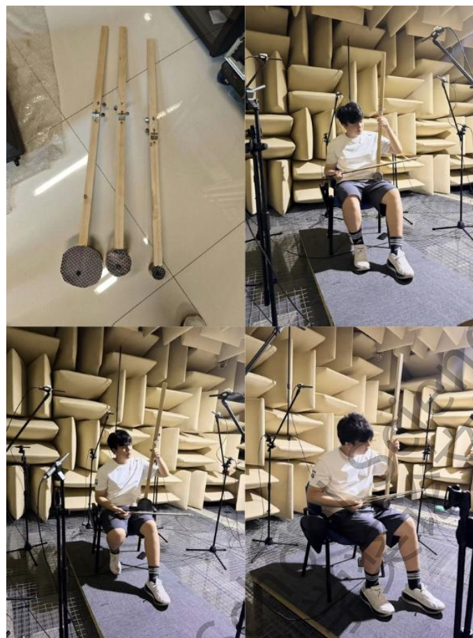
Figure 36. Three self-made gradient Huqin prototypes (large/medium/small) and test setup photo.
