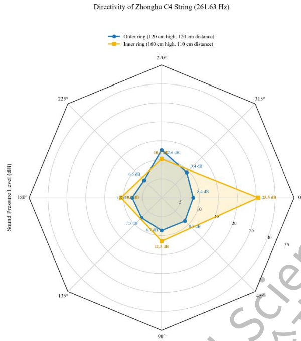
Figure 45. Absolute sound pressure level directivity of Medium Huqin at C4 (outer ring blue circles, inner ring orange squares)
