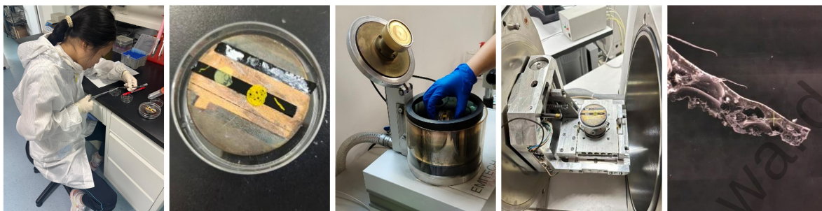
Figure 2. Process of sample preparation for SEM and microscopic morphology observation
